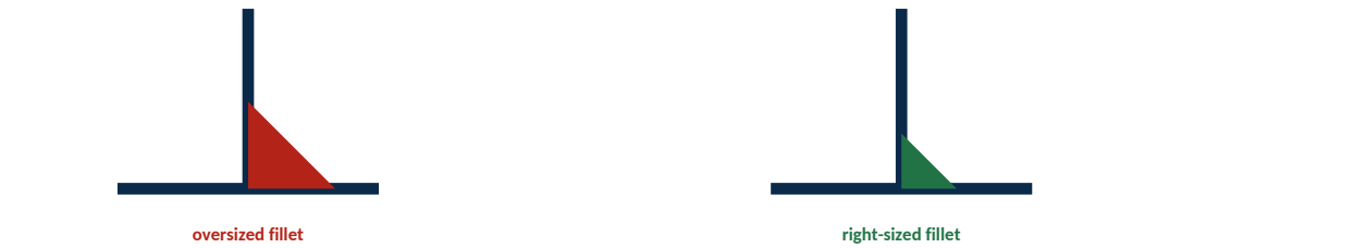
Weld size must still meet the governing design code, load path, fatigue, seal and corrosion requirements. Never reduce a weld from appearance alone.
